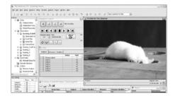
**The Observer XT** - Behavior recording for live or video-based observations. Integrated physiological measurements. Also available on handheld computers.
