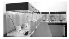
**PhenoTyper** - Video-based observation system for continuous automated monitoring of rodent behavior.
